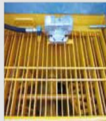
4 Hopper designed for concrete spraying
