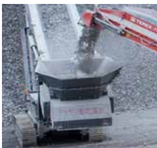
Feed Boot Liner Extension and Dust Covers
