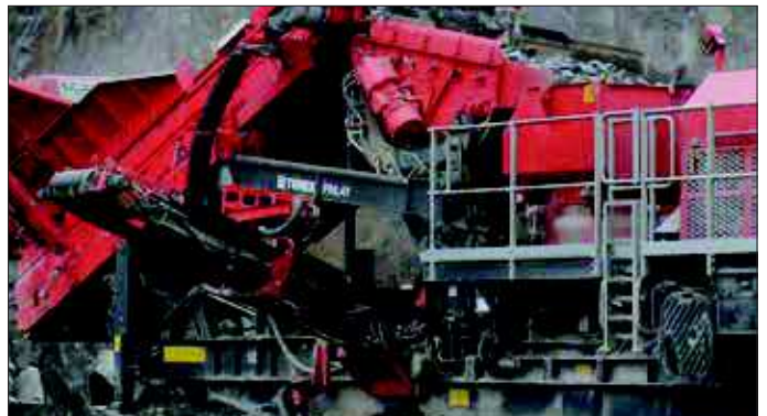
Pre-Screen & Pre-Screen Side Conveyor (Optional)
