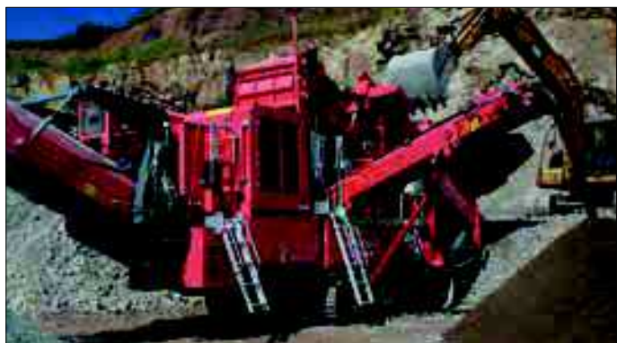
Pre-screen side Conveyor
