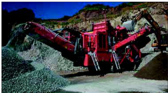
Pre-screen side Conveyor
