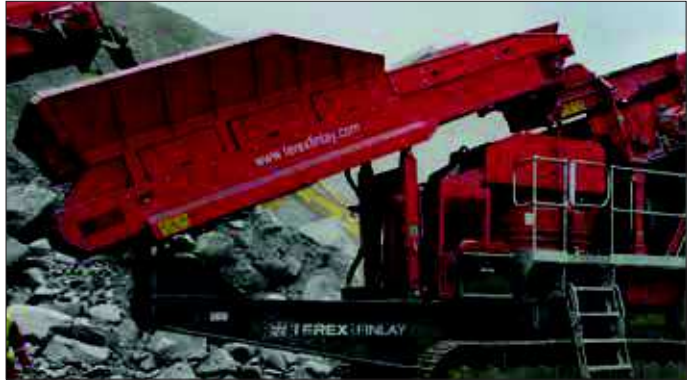
Hopper and Feeder
