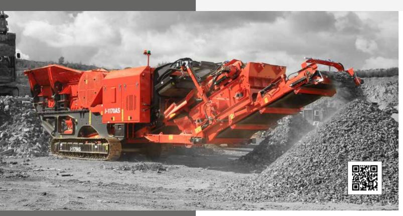
The Finlay® J-1170AS mobile jaw crushing plant provides the flexibility of a crushing and screening plant on one machine. This aggressive machine features a detachable on-board sizing screen.
