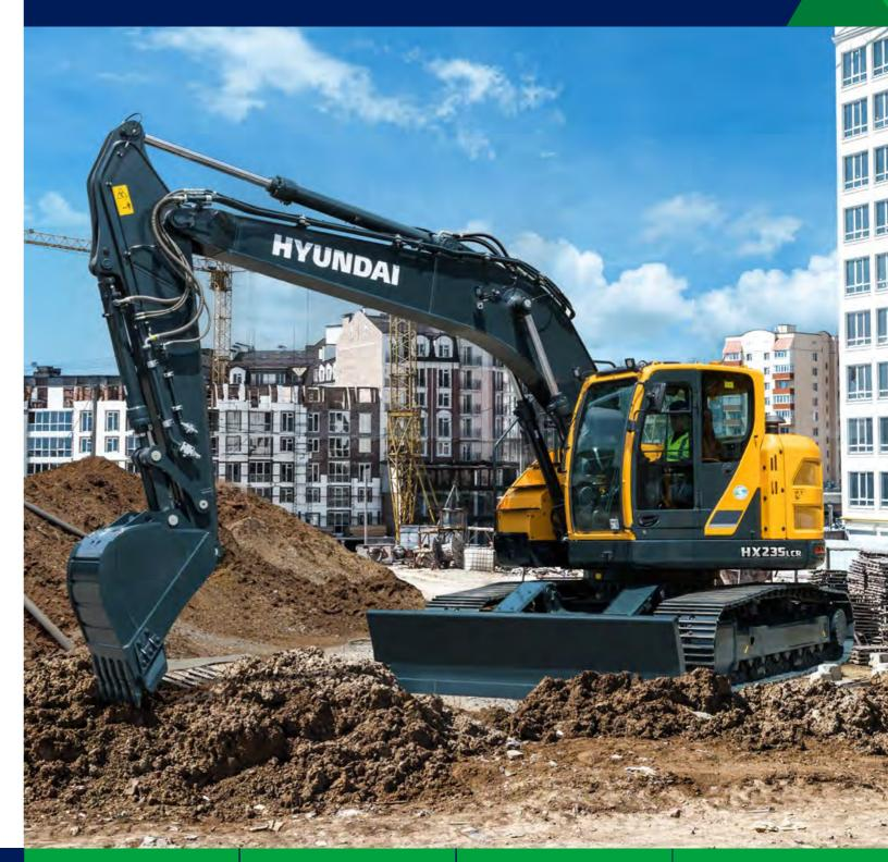
**Gross Power** 119 kW (160 HP) at 2,200 rpm **Net Power** 117 kW (157 HP) at 2,200 rpm Bucket Capacity  $0.80 \sim 1.34 \text{ m}^3$
