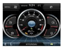
\* P(power) mode: Maximizes speed and power of the equipment for heavy load work. \* S(standard) mode: Optimizes performance and fuel efficiency of the equipment for
